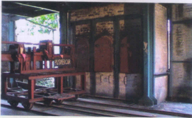
Pilot non-recovery coke oven with stamp charging facility
