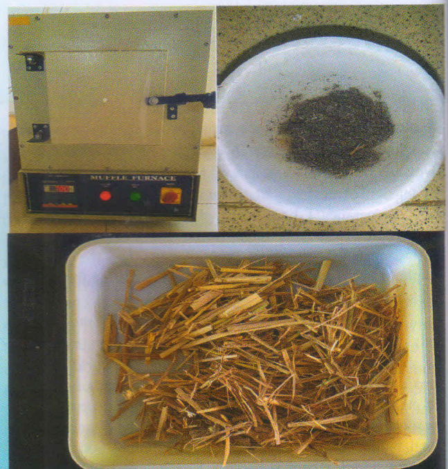
Figure 2: Clockwise from top, muffle furnace set at 700°C, the dried rice straw (RS) sample and the rice straw ash (RSA)
