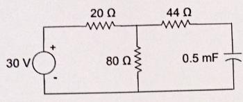
Calculate constant of the RC circuit shown in below.
