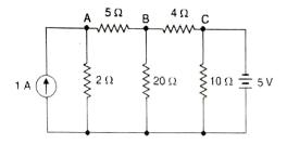
9. Calculate the current through 20 ohm resistance using thevenin's theorem. (5)
