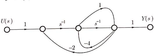
8. Indicate the overall transfer function of the system whose signal flow graph is shown in Fig.
